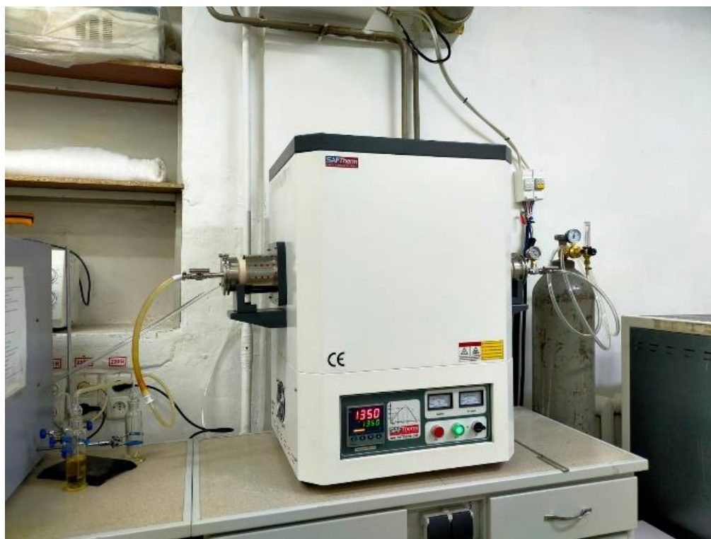
Figure 1. High Temperature Tubular Vacuum Furnace for MAX Phase Synthesis
